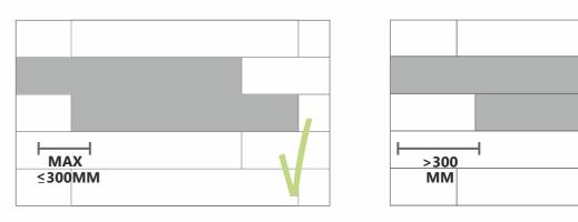
The longest side should be staggered no more than 300mm when laid in running bond.
